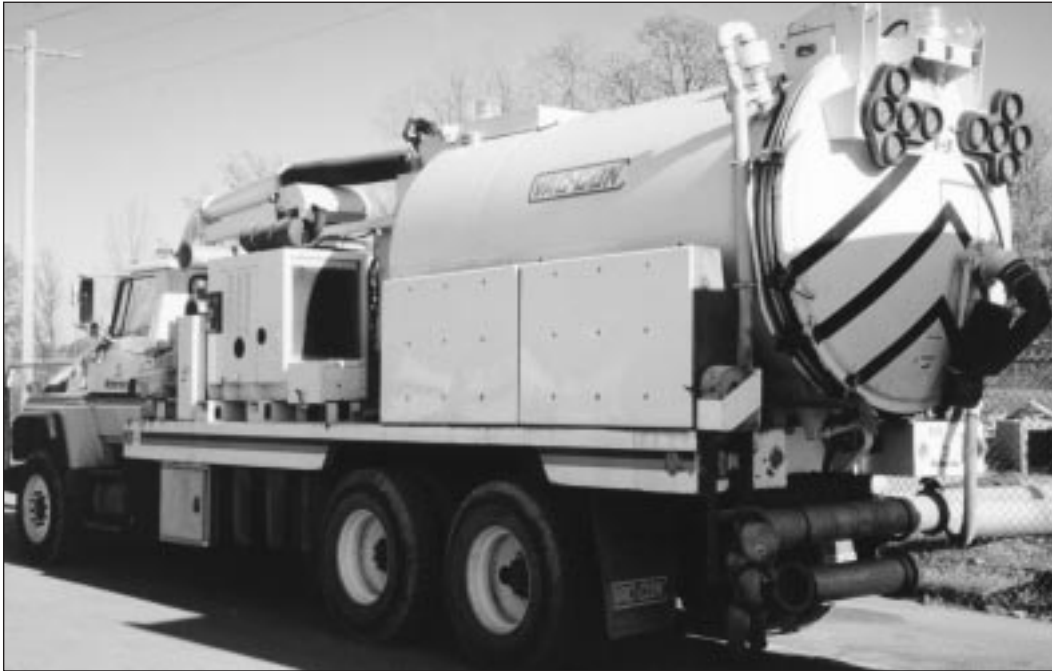
Vacuum truck for catchbasin cleaning
