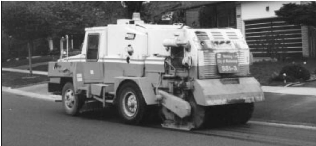
This sweeper does a good job removing heavy sediments at spring cleanup
