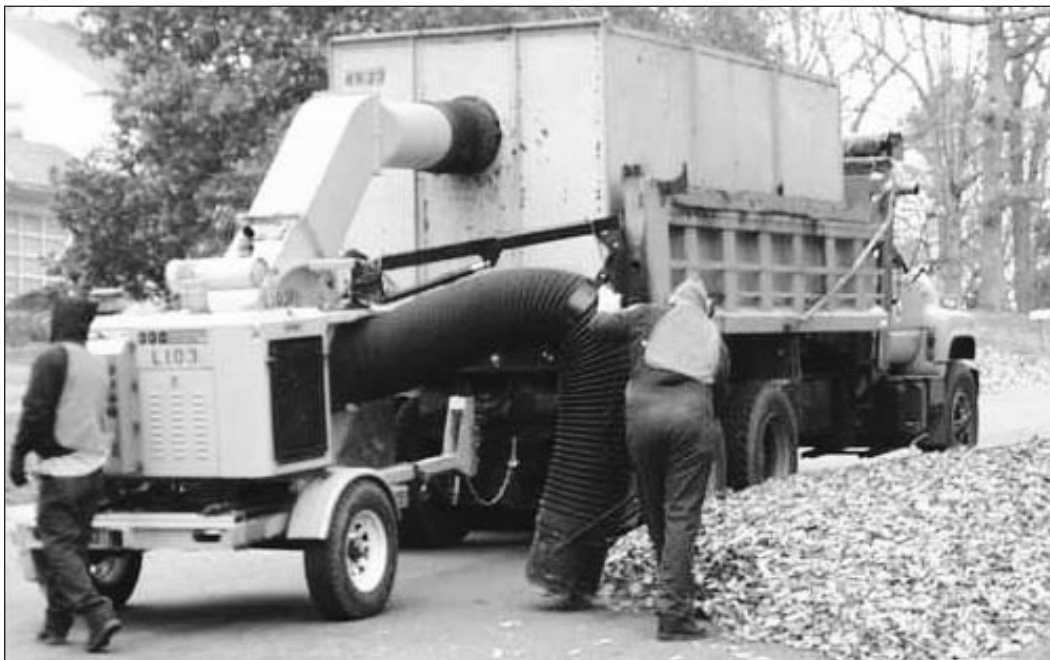
Vacuum truck and equipment for leaf removal
